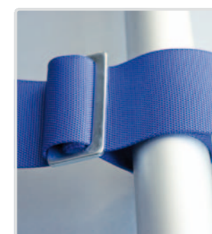
Attacco cintura a Rollbar Rollcage harness fixing
